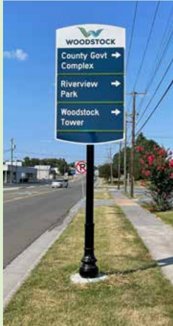
This is a sample custom trailblazer sign designed for Woodstock, Virginia. Typically, trailblazers list no more than three destinations and are designed for the size and speed of the road. The Woodstock sign system was required to go through VDOT review and approval since their streets are maintained by VDOT as are the streets in the Town of Louisa.
